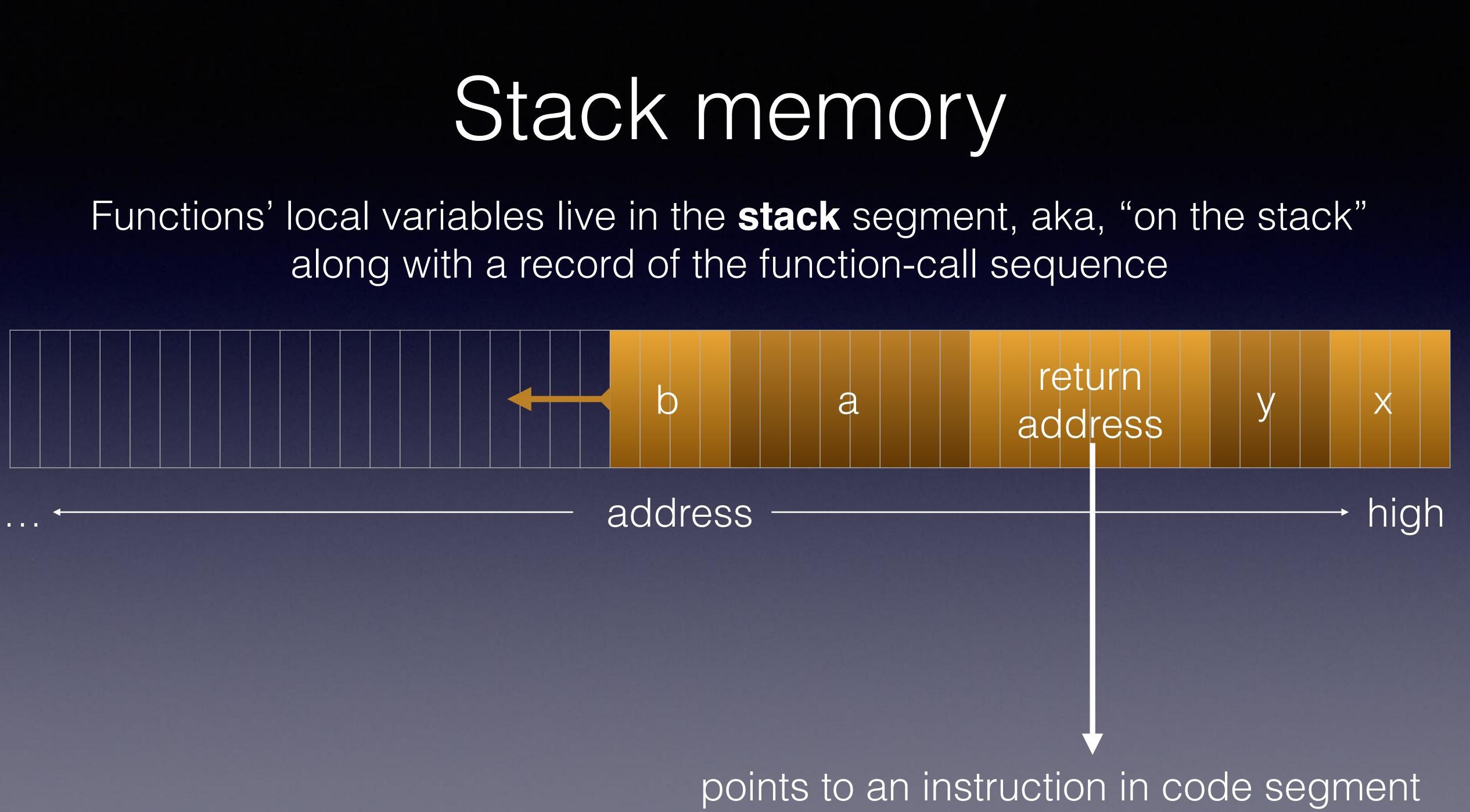
main @ 0x0000400566 - code segment x @ 0x7ffdbf396d3c has value 2 y @ 0x7ffdbf396d38 has value 5 change @ 0x0000400645 - code segment a @ 0x7ffdbf396d18 has value 2 at 0x7ffdbf396d3c b @ 0x7ffdbf396d14 has value 5 main @ 0x0000400566 x @ 0x7ffdbf396d3c has value 99 y @ 0x7ffdbf396d38 has value 5
