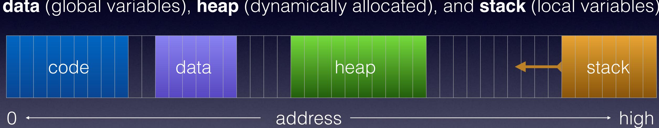
Not all addresses will be used; and different compilers and operating systems may lay out the four segments differently
