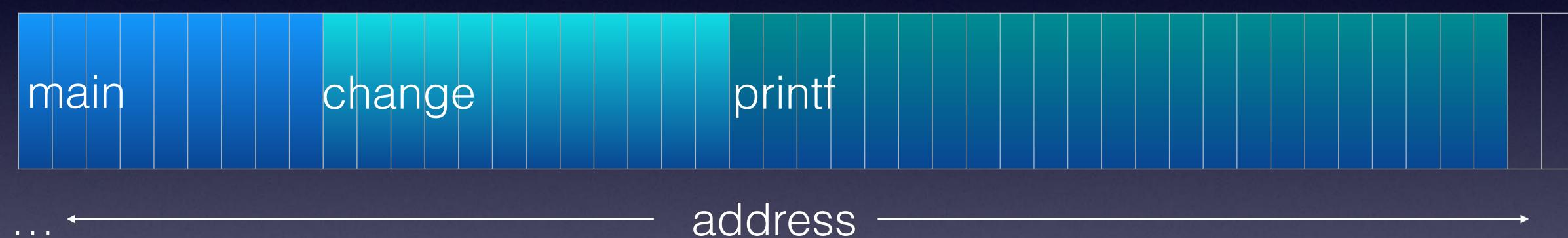
See example: pointer2.c Again, the code segment is not necessarily in low memory.
