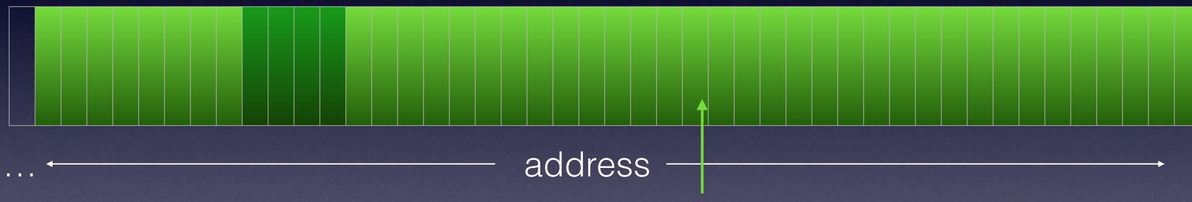
After free(hello) the heap manager thinks the space is now unallocated and can be used to support future malloc() calls. If we keep and re-use the hello pointer, bad stuff happens!
