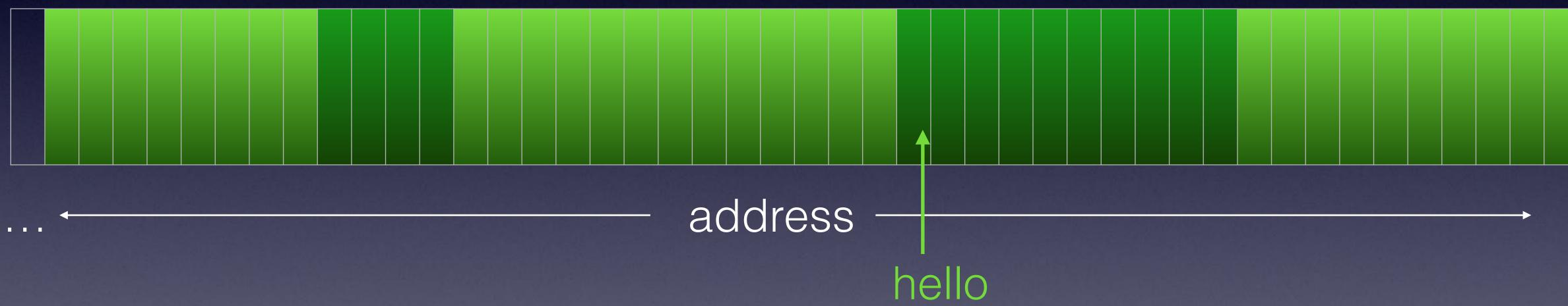
The heap manager allocates 10 bytes and returns the address, which we save in the pointer variable hello.
